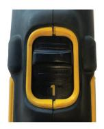
STEP 4: Always use setting #1 when using the recommended right angle battery drill.
